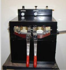
proper clamping force. Large clamping jaws to reduce deflection at high clamp force and reduce heat build up during high current flow. Grease fittings are placed on all bearings to allow simple maintenance of moving parts.
